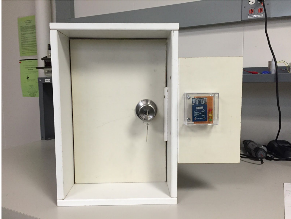
Figure 13 RFID module end product installed on door model
