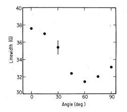
FIG. 2. Resonance linewidth versus magnetic field orientation for a Ag:0.1-at.%-Er film on fused quartz, at 1.5 K. The angle plotted is  $\theta'$ , between the magnetic field and the normal to the film. The significance of the angular dependence is discussed in the text.
