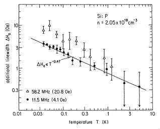
FIG. 7. Additional linewidth of Si:P doped to  $n = 2.05 \times 10^{18}$  cm<sup>-3</sup> as a function of temperature at two values of the magnetic field. The solid line is a guide to the eye. It suggests a critical behavior at T = 0.
