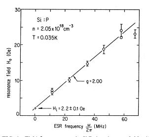
FIG. 2. Field for resonance in Si:P doped to  $n=2.05\times10^{18}$  cm<sup>-3</sup> as a function of the ESR frequency at T=35 mK. The g=2.00 slope indicated by the solid line is that expected of noninteracting donors in Si. The intersection at  $\omega/2\pi=0$  indicates the presence of a local field directed opposite to the applied field. This local field is interpreted as due to interactions among the donor spins.
