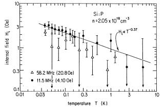
FIG. 8. Internal fields as a function of temperature for Si:P doped to  $n = 2.05 \times 10^{18}$  cm<sup>-3</sup> at two values of the applied field. The solid line is a guide to the eye.
