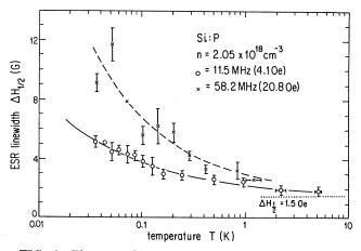
FIG. 4. Electron-spin-resonance linewidth in Si:P doped to  $n = 2.05 \times 10^{18}$  cm<sup>-3</sup> as a function of temperature for two resonance frequencies. The lines are a guide to the eye.
