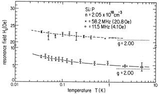
FIG. 3. Field for resonance in Si:P doped to  $n = 2.05 \times 10^{18}$  cm<sup>-3</sup> as a function of temperature for two resonance frequencies. The solid and dashed lines are a guide to the eye. The increase in  $H_0$  with decreasing temperature indicates the temperature dependence of the local field.
