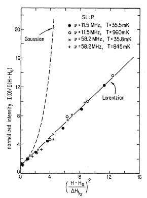
FIG. 5. Normalized line shape of the ESR absorption in Si:P doped to  $n = 2.05 \times 10^{18}$  cm<sup>-3</sup> for two frequencies and two temperatures. The solid line corresponds to a Lorentzian shape [Eq. (1)] and the dashed line represents a Gaussian. The close agreement to the Lorentzian form is an indication that hysteresis in the cycling of the local field is negligible, and that the line shape is determined by exchange and/or motional narrowing.
