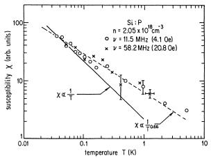
FIG. 6. Temperature dependence of the susceptibility of a sample of Si:P doped to  $n = 2.05 \times 10^{18}$  cm<sup>-3</sup> at two different ESR frequencies. The data from the two different frequencies are both displayed on an arbitrary susceptibility scale. The substantial deviation from the Curie-law behavior indicated by the solid line is attributed to the interactions among the spins, and the dashed line indicates the static measurements reported in Ref. 5.
