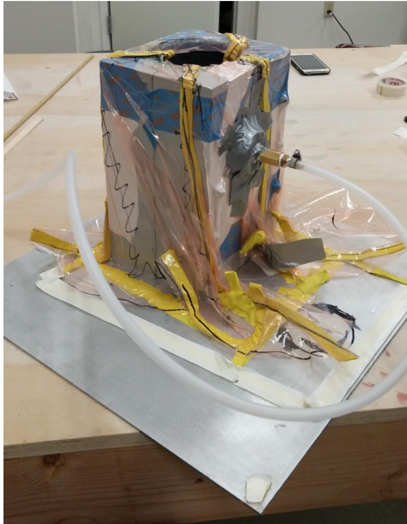
Figure 28: Vacuum bag setup for nose cone layup; notice the bag has been seamed along the diagonals, in order to approximate the interior curvature of the mold. Additionally note the multiple dog ears in order to guarantee vacuum seal.
