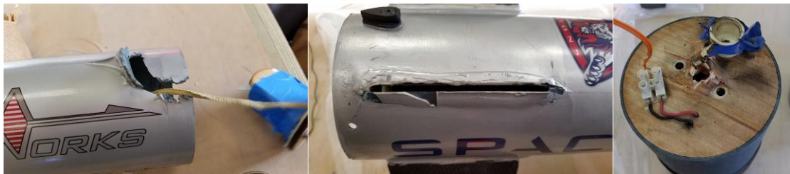
Figure 25: Damage caused by deployment of main chute at high velocity
