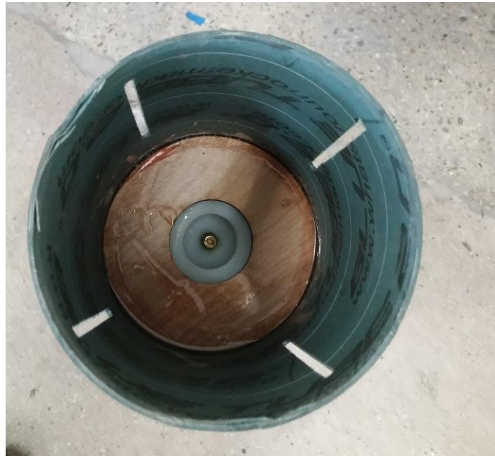
Figure 5: 3/16" laser cut plywood centering ring.
