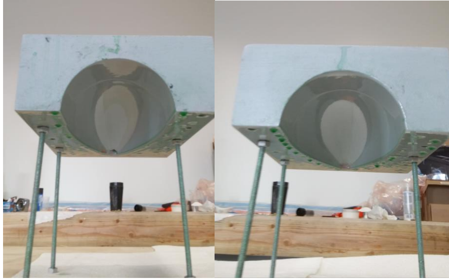
Figure 27: Detail view of primary mold surfaces of nose cone mold during PVA drying.
