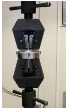
Figure 18: Engine block tensile testing setup
