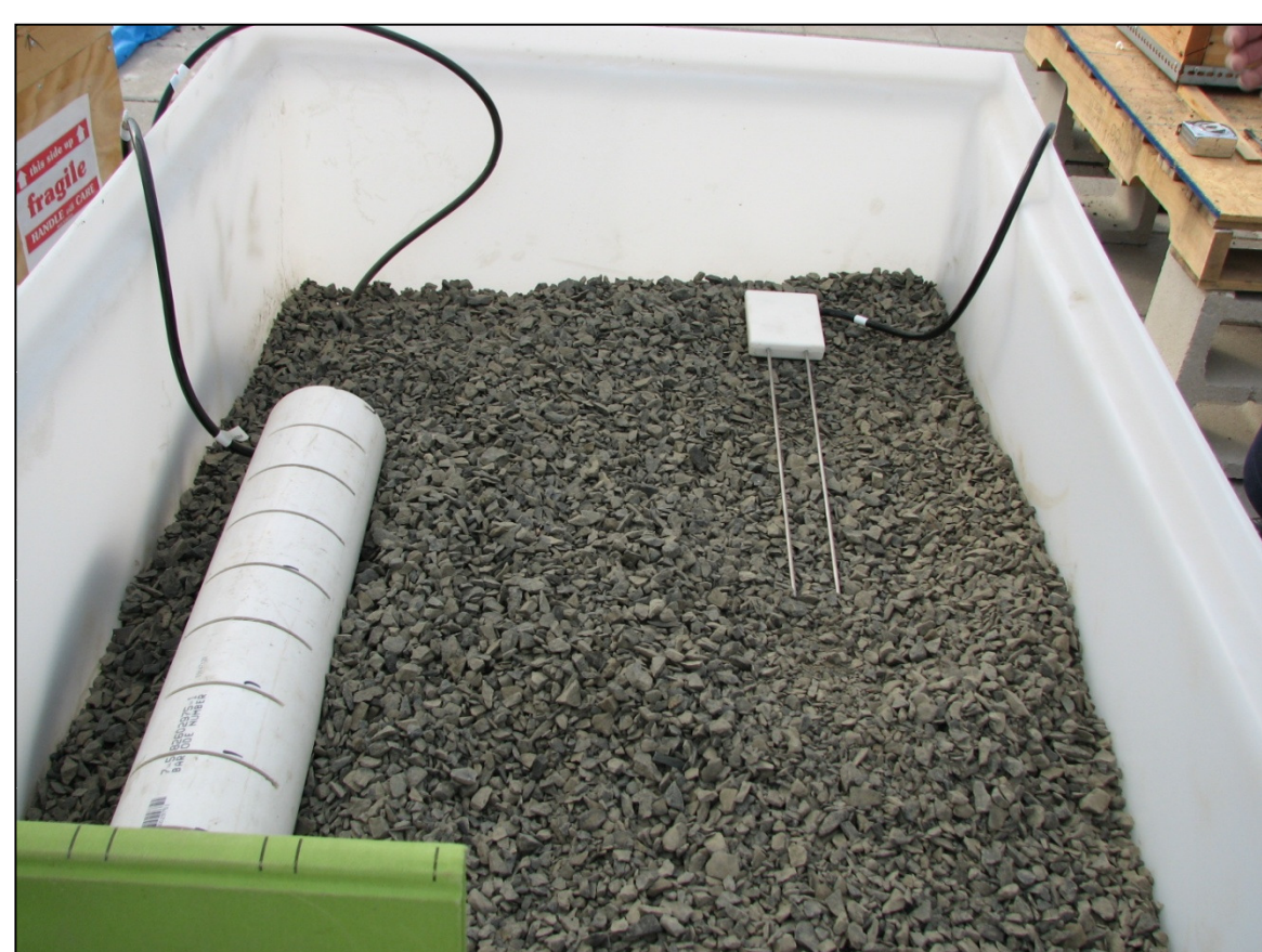
Figure 1. The response of TDRs in 5/8" diameter gravel with protective PVC housing (left) and without housing (right) were studied at the bench scale under saturated conditions.
