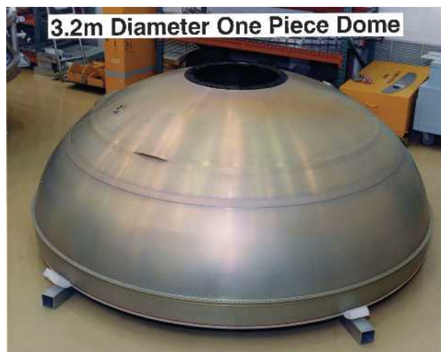
Fig. 1 One-piece dome for a cryogenic tank (2219 alloy)
