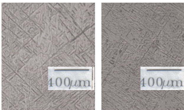
Fig. 7 Long (a) and rolling (b) direction views of the wrought Ti-6Al-4V microstructure after being annealed (beta-aged) at 865 °C
