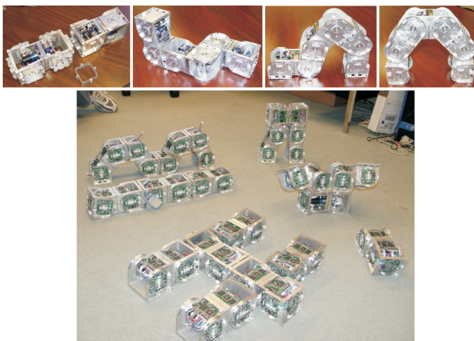
Fig. 8. Example configurations of robotic stem cells based on SuperBot modules.
