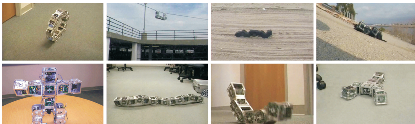
Fig. 9. Multifunctional examples of robotic stem cells based on SuperBot modules. From top-left to bottom-right: (1) a rolling track composed of six modules, (2) a rope climber of three modules, (3) an “inchworm” formed by four modules, (4) a slope climber with four modules, (5) a “humanoid” formed by six modules, (6) a sidewinder “snake” configured by seven modules, (7) a “caterpillar” of three modules and (8) a “scorpion” with four modules.
