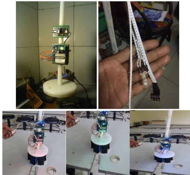
Gambar 4. Visualisasi Sinyal Transmisi Data, (atas kiri-kanan) Mikro-Kontroller dan Sensor Atmosfer Serta Lampu Indikator, (bawah) Lampu Indikator Untuk Proses Pencarian Sinyal. Figure 4. Visualization of Data Transmission Signals (top left-right) Micro-Controller and Atmospheric Sensor and Indicator Light, (below) Indicator Lamp For Signal Search Process.
