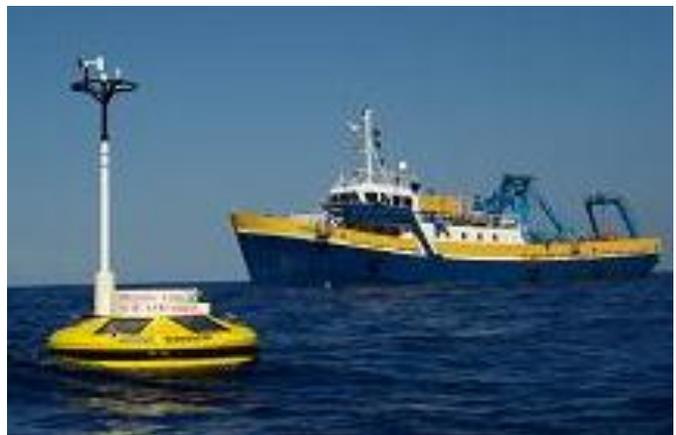
Gambar 4. *Wave Scan Tsunameter buoy*
