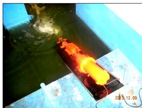
Gambar 3. Pengujian motor di kolam Figure 3. Motor test arrangement
