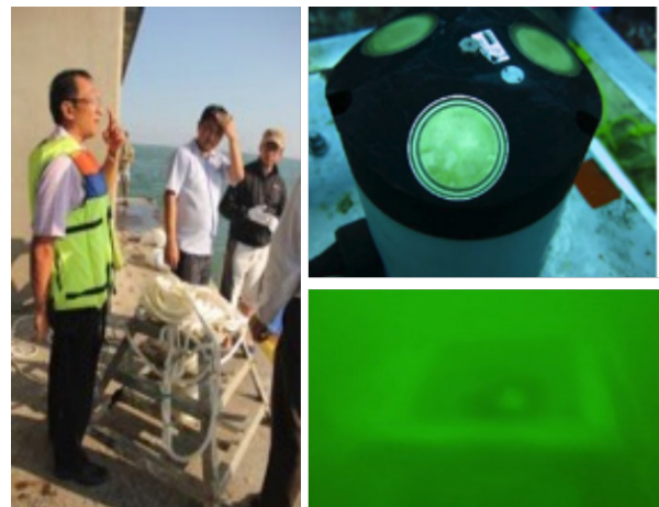
Figure 5. ADCP setting and placement on the sea bottom of the study area.
