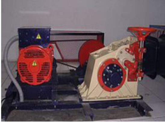
Gambar 2.1 Mikrohidro Tipe Cross flow
