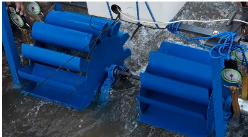
Figure 3. Undershot type waterwheel
