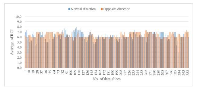
Fig. 4. Nomogram of RCI value on the Caruban-Ngawi road segment (all data)
