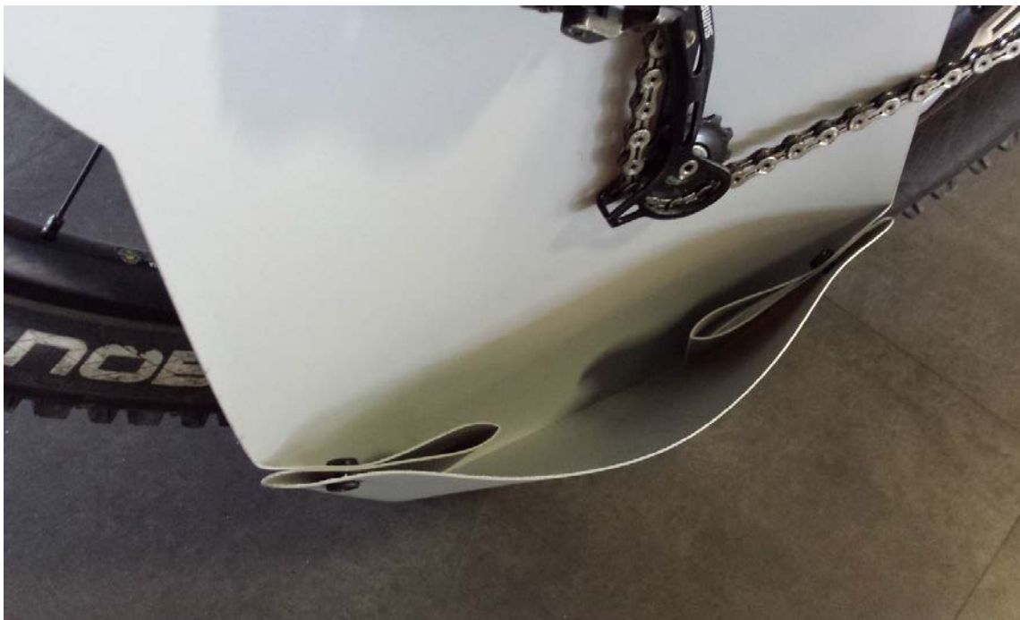
Figure 12: Version 5 folded pocket close up showing the excess material of the fold.
