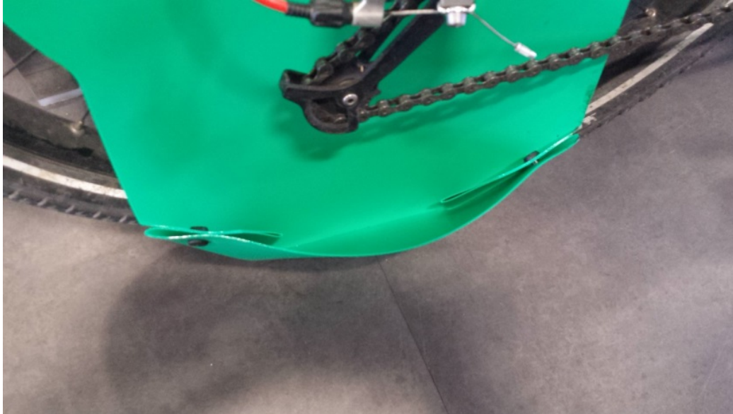
Figure 13: Version 6 folded pocket close up showing the reduction of the excess material of the fold.
