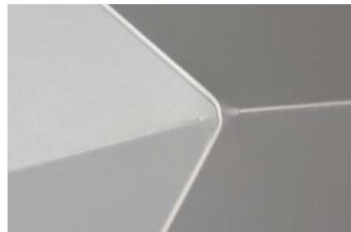
Figure 10: Close up of laser scoring fold.
