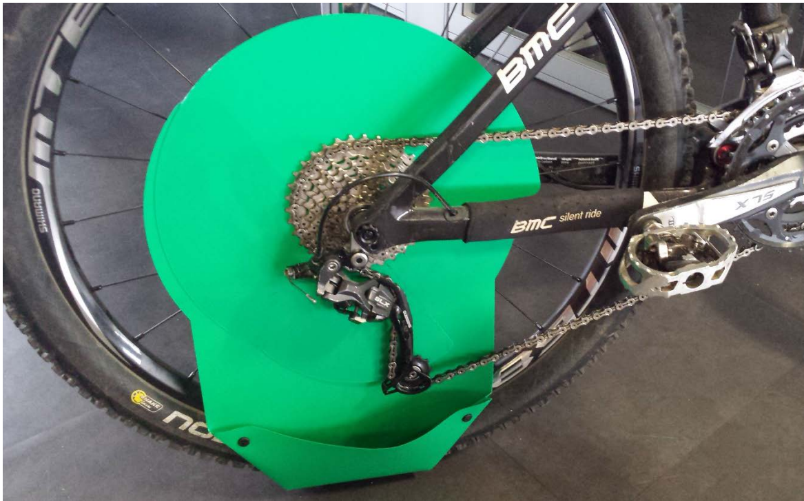
Figure 17: Version 7 closed to protect the disc brakes and ready for use.
