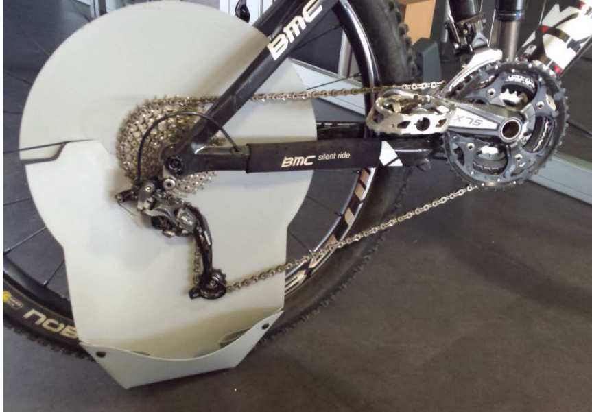
Figure 11: Version 5 under testing showing the split line hooking over the spokes.
