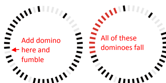
Figure 2 shows how fumbling one domino affects a line of dominoes in one direction until there is a space.
