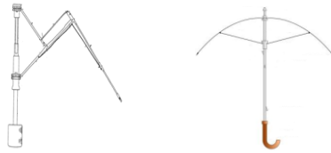
Figure 1: Illustrations of the two types of umbrella discussed in this paper. The diagram on the left shows the structure of a typical jointed umbrella (adapted from source [6]), whereas the other shows a solid structure (adapted from source [7]). The jointed structure is more susceptible to collapse.
