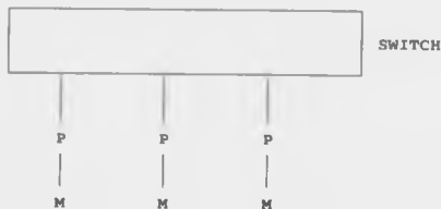
Fig. 3.5: Distributed-memory MIMD architecture.
