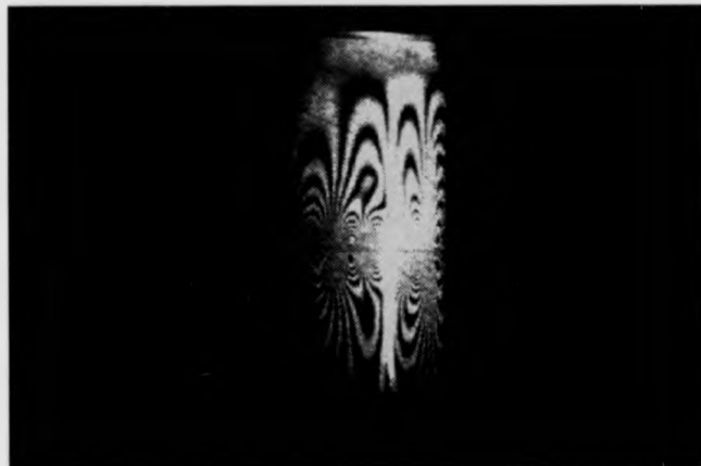
Figure 6.1: Double-exposure hologram of a stressed aluminium can (image size 512 \times 512 ).
