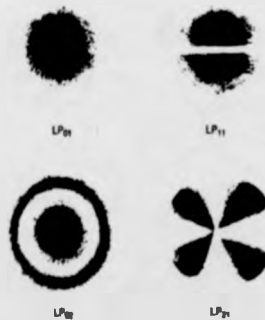
Figure 4.9: The irradiance pattern in the output of the fibre.
