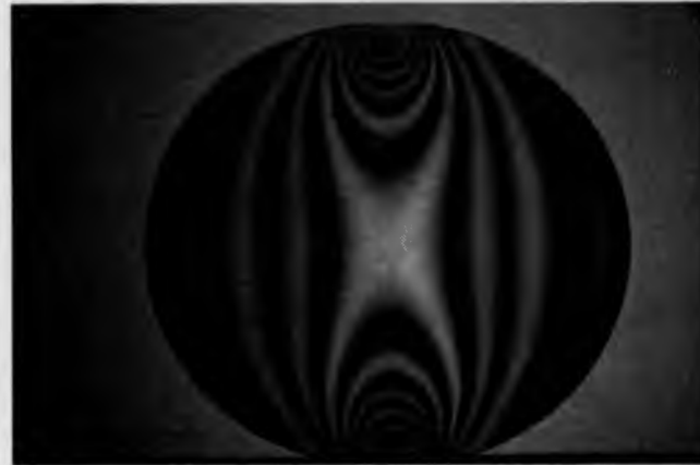
Figure 8.5: Isochromatic fringe pattern of light field obtained using circular polariscope (image size 512 \times 512 ).
