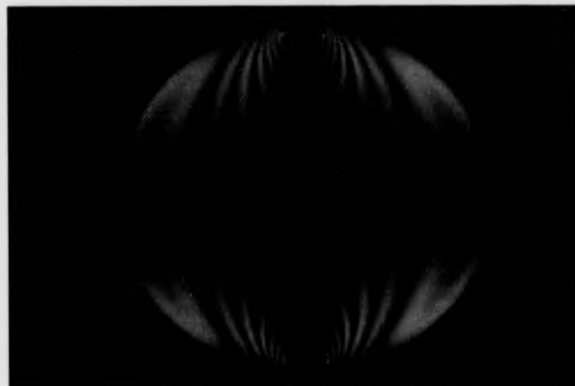
Figure 8.2: Isoclinic fringe pattern generated by a plane polariscope (image size 512 \times 512 ).
