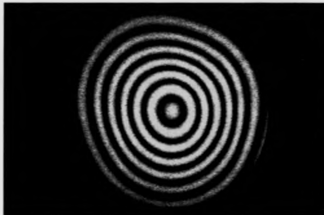
Figure 2.15: Example of double-exposure hologram showing the deformation of a silicon wafer under central loading (image size 512 × 512).
