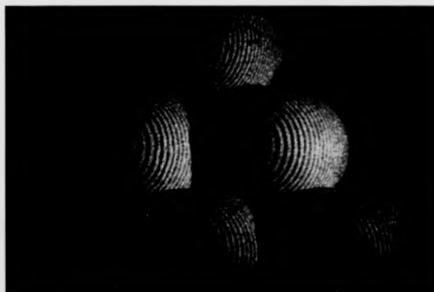
Figure 5.29: Holographic contouring fringes on the same balls as in Figure 5.28, but with different viewing direction (image size 512 × 512).
