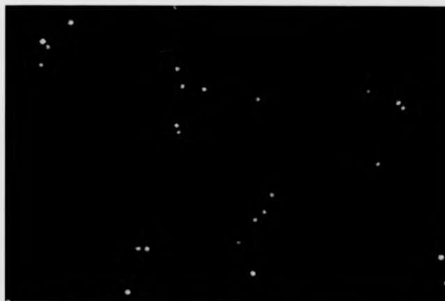
Figure 2.19: Reconstructed holographic particle image obtained by CCD camera using diffraction limited lens (image size 512 \times 512 ).
