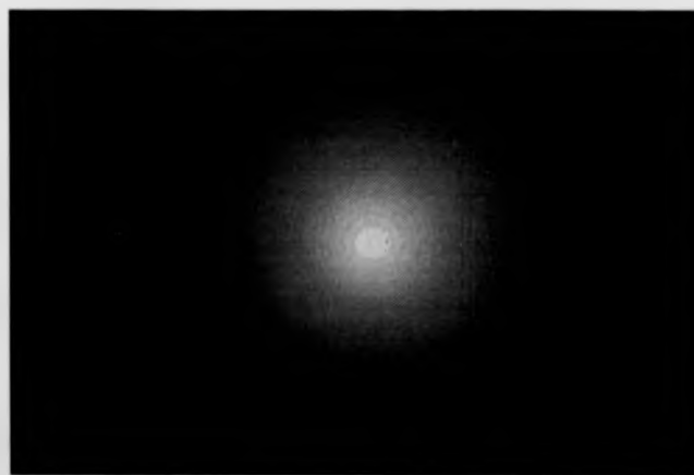
Figure 7.25: Normalised grey scale plot of deformation produced by unwrapping procedure, before correction for non linearity of carrier fringes (image size 512 \times 512 ).
