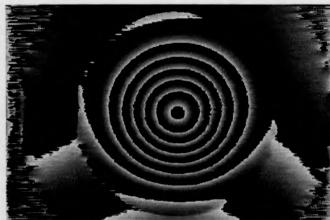
Figure 7.23: Wrapped phase map generated by FFT technique (image size 512 \times 512 ).
