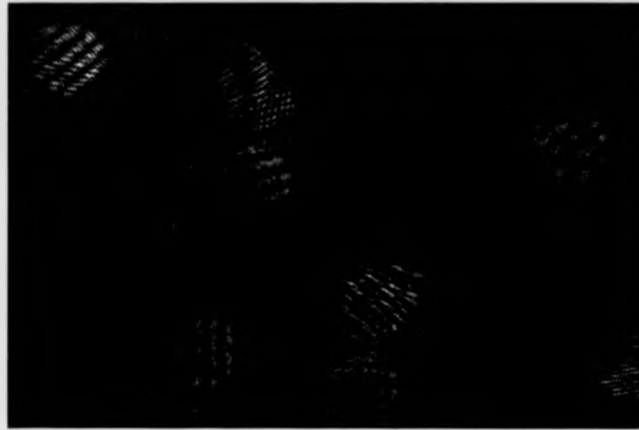
Figure 2.20: Youngs fringe pattern of holographic particle image obtained by defocus of diffraction limited lens (image size 512 \times 512 ).
