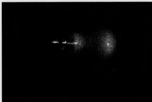
Figure 5.18: Holographic contouring fringes on a light bulb (image size 512 × 512).
