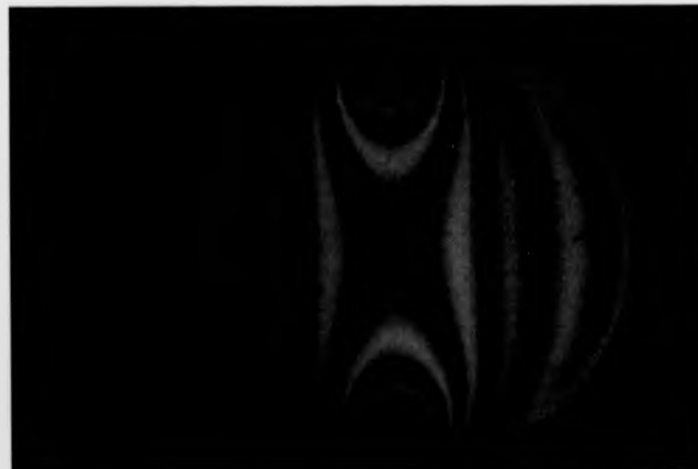
Figure 8.4: Isochromatic fringe pattern of dark field obtained using circular polariscope (image size 512 × 512).
