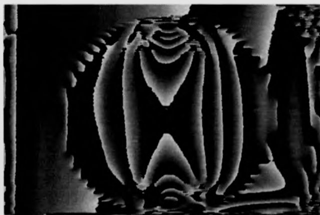
Figure 8.31: Wrapped phase map of a circular disk with errors (image size 512 \times 512 ).
