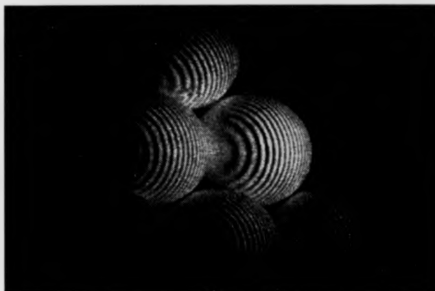
Figure 5.28: Holographic contouring fringes on the balls (image size 512 × 512).
