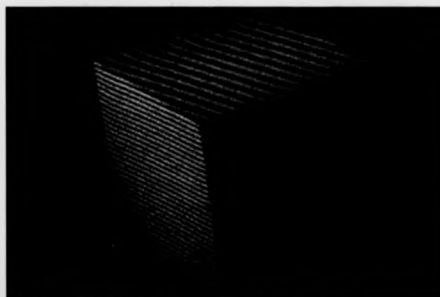
Figure 5.19: Holographic contouring fringes on a cube (image size 512 × 512).
