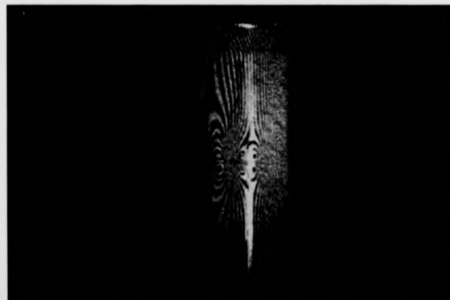
Figure 6.2: Double-exposure hologram of a deformed aluminium can with carrier fringes (image size 512 \times 512 ).
