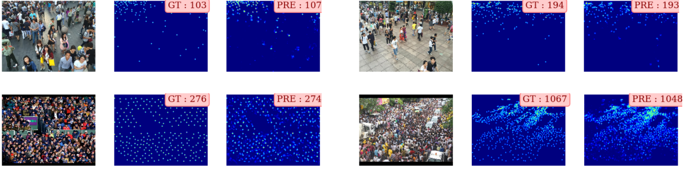
Figure 5: Qualitative results on ShanghaiTech Dataset. For each group of images, pictures in the middle and on the right are corresponding ground truth and estimated density map of the image on the left, where the number on the top right corner indicates the ground truth (GT) and the estimated number of people (PRE) respectively. It can be seen that SDANet has a strong adaptability to different density levels with a error less than 4%.
