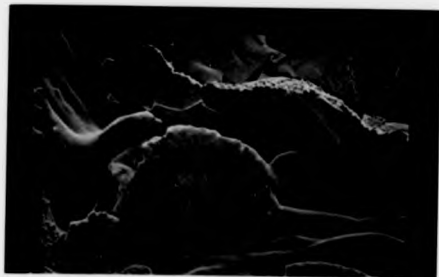
Figure 41 Large cracks on the flank face of KYON 2000 after machining EN8 at the speed of 700 m/min
