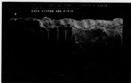
Figure 69 General view of KYON 2500 tool after machining EN24 at a speed of 400 m/min
