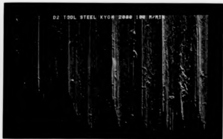
Figure 93 Showing ridges on the worn flank face of KYON 2000 when machining D2 tool steel at a speed of 100 m/min
