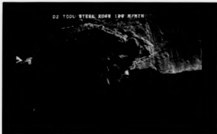
Figure 81 Showing the extent of flaking at the cutting edge of KO60 tool after machining D2 tool steel at a speed of 100 m/min
