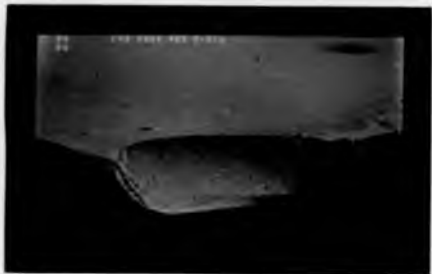
Figure 33 Showing general view of fracture surface of mixed oxide ceramic tool (KO90) when machining EN8 steel at speed of 700 m/min
