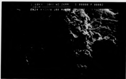
Figure 72b Showing severe chipping and plucking after machining EN24 with KYON 2000 at a speed of 100 m/min
