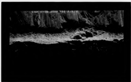
Figure 37 Severe chipping at the cutting edge of Kyon 2500 tool when machining EN8 steel at the speed of 700 m/min
