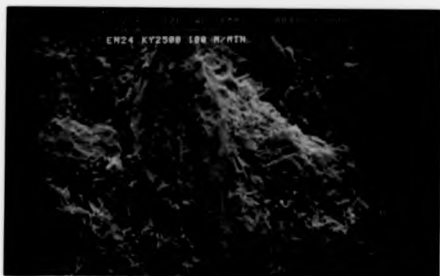
Figure 71 Showing cracks after machining EN24 with KYON 2500 at a low speed of 100 m/min
