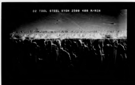
Figure 89 Showing a combination of flaking at the cutting edge and plucking and cracks on the flank face
