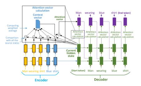
Fig. 4: Encoder decoder framework of sentence generation with attention mechanism. All the hidden states of the encoder are compared with current state of decoder to find weights, which are then used to find context vector by computing a weighted average. Subsequently, the computed context vector is combined with current state of the decoder to generate attention vector for feeding to the next time step.
