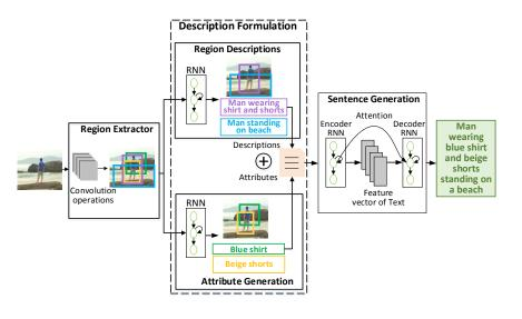
**Fig. 1:** Architecture overview. Object regions are extracted by region extraction module. Region descriptions and object attributes are then generated from these extracted regions. Afterwards, sentence generation component joins all the produced region descriptions and attributes to form a detailed descriptive sentence
