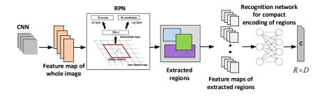
Fig. 2: Region extraction block. CNN extracted features are fed to RPN for region extraction.
