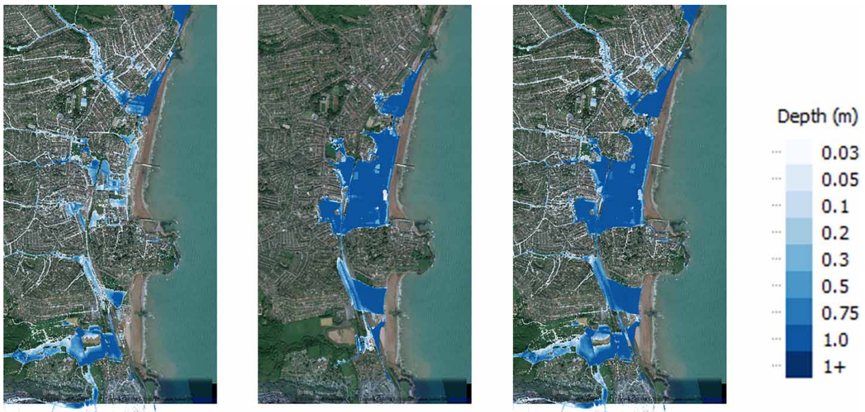
Figure 8 | Flood extents of a 1 in 100-year return period pluvial event (left) and a 1 in 200-year return period overtopping event (centre), and combined 1 in 50-year pluvial and coastal overtopping event (right), each for the 50 years of climate change scenario.
