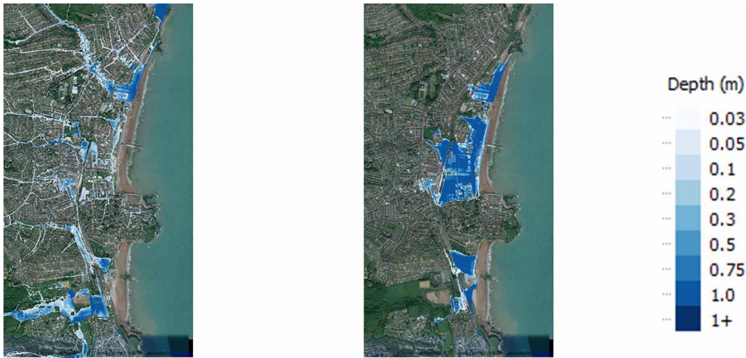
Figure 7 | Flood extents of a 1 in 100-year return period pluvial event (left) and a 1 in 200-year return period overtopping event (right) for the present scenario.
