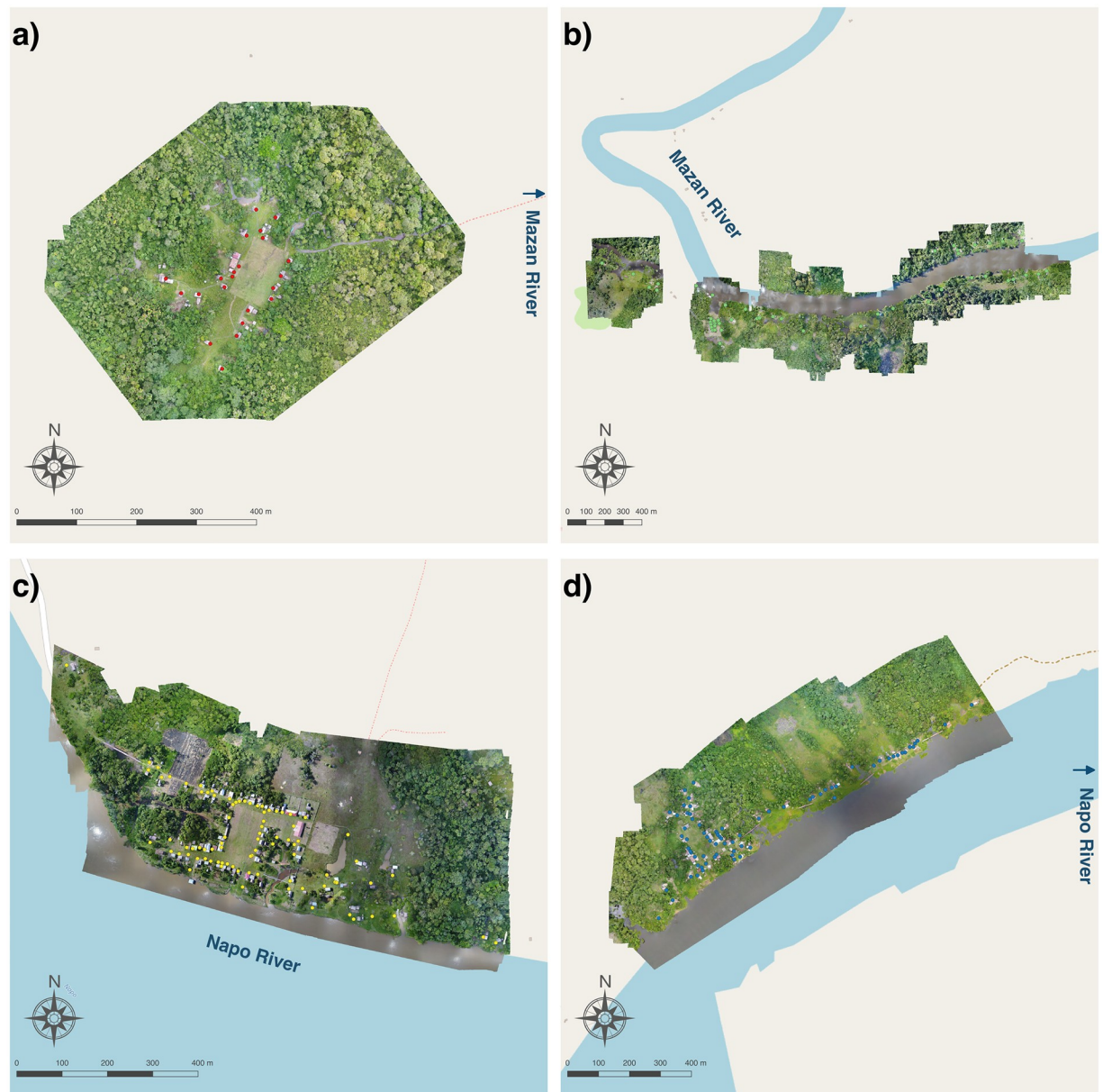
Fig 2. Orthomosaics of the communities of (a) Visto Bueno, (b) Libertad, (c) Salvador, (d) Urco Mirañó. Orthomosaics were constructed in AgiSoft Photoscan Pro ( https://www.agisoft.com ) and mapped in QGIS. The basemaps were produced in QGIS based on public geographic data from OpenStreetMap ( www.openstreetmap.org ).
