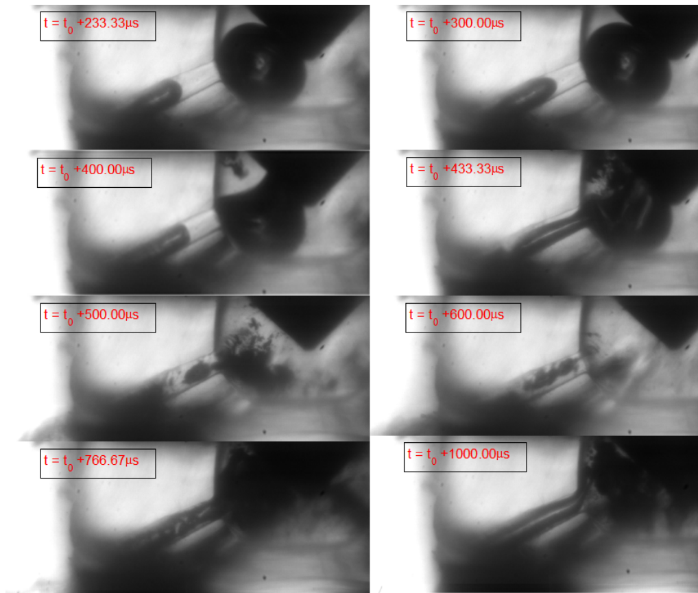
Figure 1: Experimental results. Time sequence of a pilot injection transparent nozzle tip visualisation.
