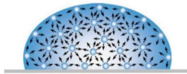
Figure 2. 3 Droplet formation on a surface due to the unbalanced forces of liquid molecules. Figure reproduced from reference 2. 2
