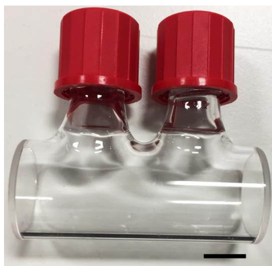
Figure 5. 9 Gas-tight glass reaction vessel used for the photocatalytic hydrogen evolution experiments. (Scale bar is 1 cm).
