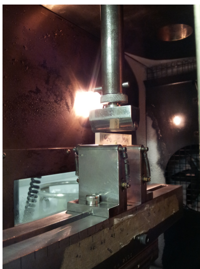
Figure 6.16: Close-up of low temperature SENB setup
