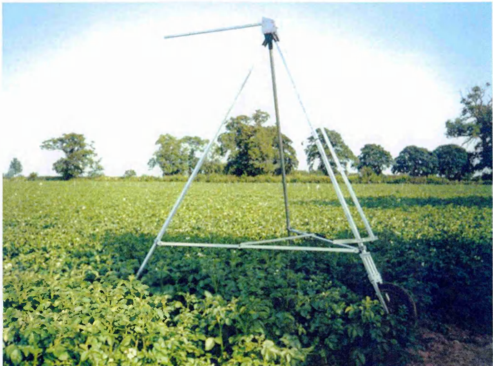
Plate 2.5. Mobile gantry designed to collect field spectra from an elevation of 4m.
