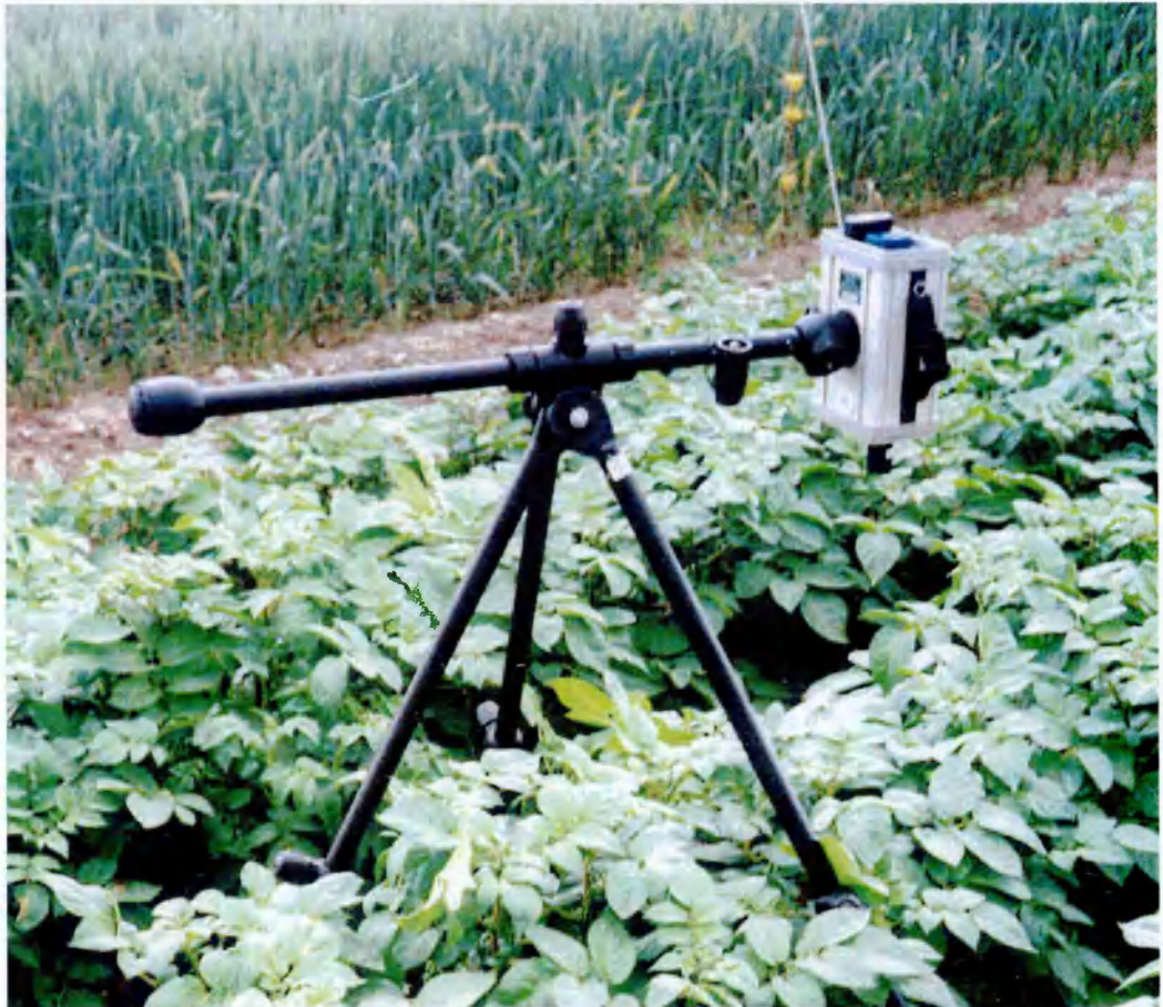
Plate 2.2. GER1500 spectrometer positioned over a target plant of the 2000 field experiment.
