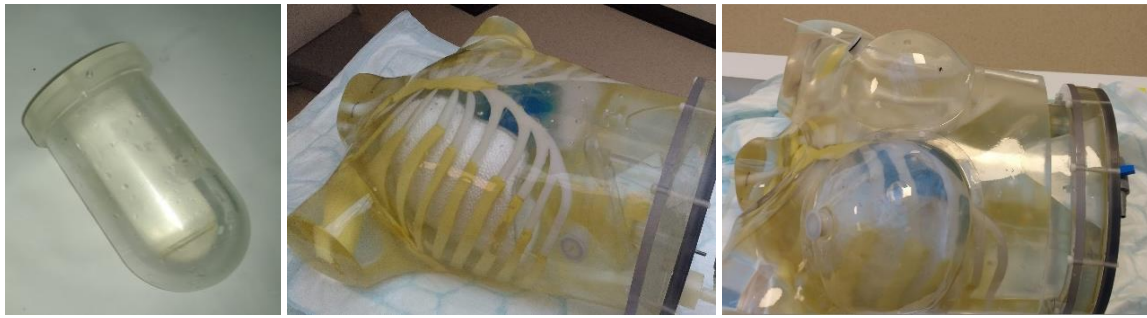
Figure 1: Anthropomorphic torso phantom (centre), with in-house replacement LV insert (left) and additional PMMA chest plate and water filled breasts (right)
