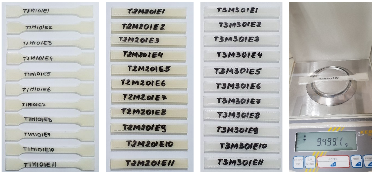
Figure 1: Example of coded specimens – a) tensile test specimens printed horizontally from M1; b) flexural test specimens printed normal from M2; c) Charpy impact test specimens printed normal from M3; d) weighing of tensile test specimen printed horizontally from M4
