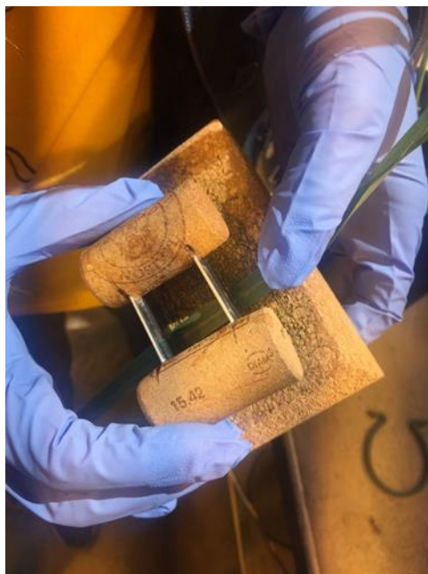
Figure 3: Image depicting the razor blade and cork apparatus used to collect leaf samples. The samples taken in the image was the first sample collected from this leaf, 5 cm from the leaf tip
