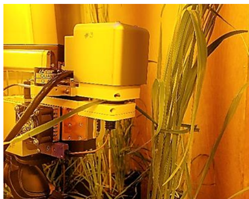
Figure 2: Image depicting the LI-6400xt clamped onto a leaf with the fluorometer head attachment
