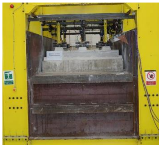
Figure 2 – Slab track tests in GRAFT II at Heriot-Watt University
