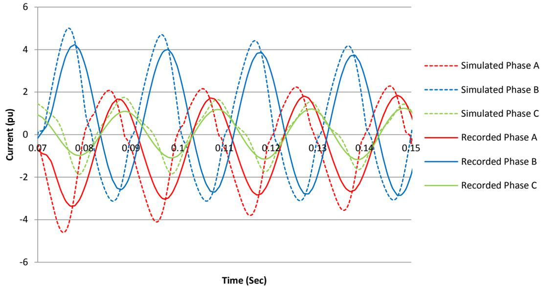
Fig. 8 Simulated current waveforms calculated using the identified generator/turbine parameter values after the 1<sup>st</sup> stage of the process compared with the recorded transient currents
