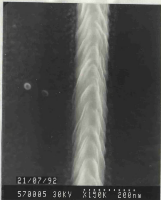
Figure 4.8.21 - SEM Micrograph of 120nm Pyramidal Gate
