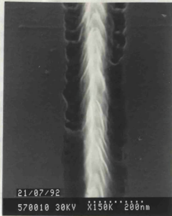
Figure 4.8.22 - SEM Micrograph of 80nm Pyramidal Gate
