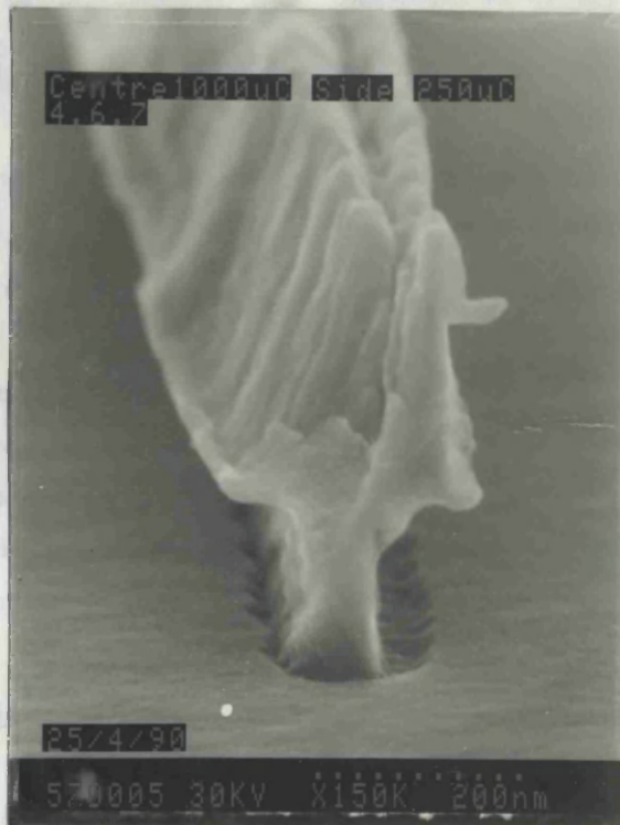
Figure 4.8.26 - SEM Micrograph of 100nm T-Gate on a Planar Substrate
