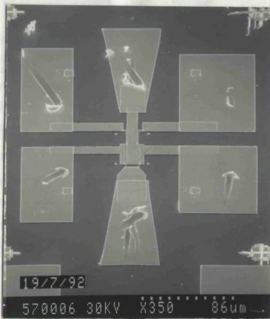
Figure 4.8.13 - SEM Micrograph Overview of Gate Resistance PCM
