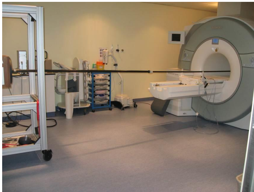
Figure 1.4: Mechanical method of MRE wave excitation at The University of Edinburgh, Clinical Research Imaging Centre: sub-woofer, piston and MRI scanner.
