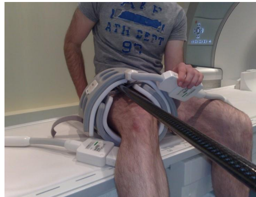
c) Thigh actuator, piston and flex coil
