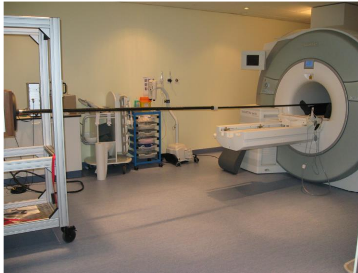
a) MRE set-up; Subwoofer, piston and MRI scanner
