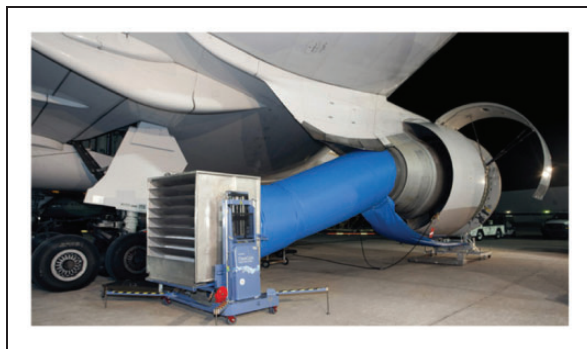
Figure 4. On-wing compressor washing with capture of effluents. 8
