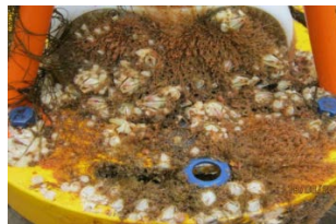
Figure 3: ADCP after 2 years under water [7]
