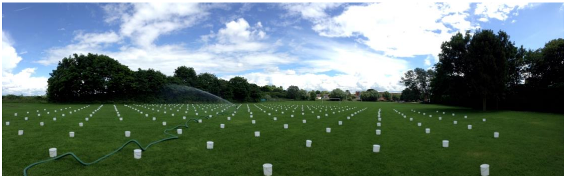
Figure 5.8 Panoramic view of the catchcan grid during an irrigation test
