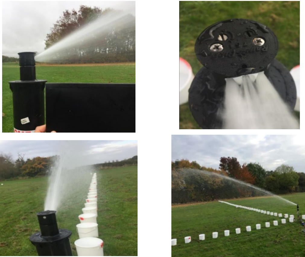
Figure 5.29 Jet formation in the RainBird 751 sprinkler fitted with the nozzle #28.
