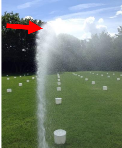
Figure 5.22 Distortion of the sprinkler jet due to wind.
