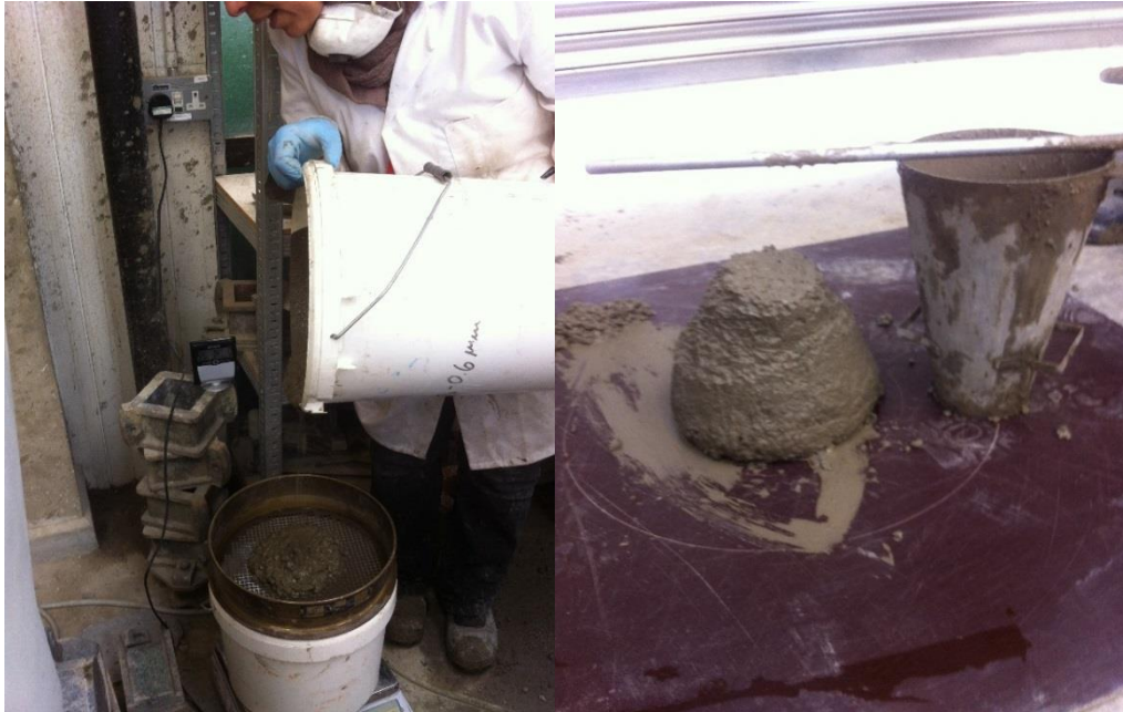
Figure 3-6 Sieve stability test (a) Slump test for NC mixes (b).
