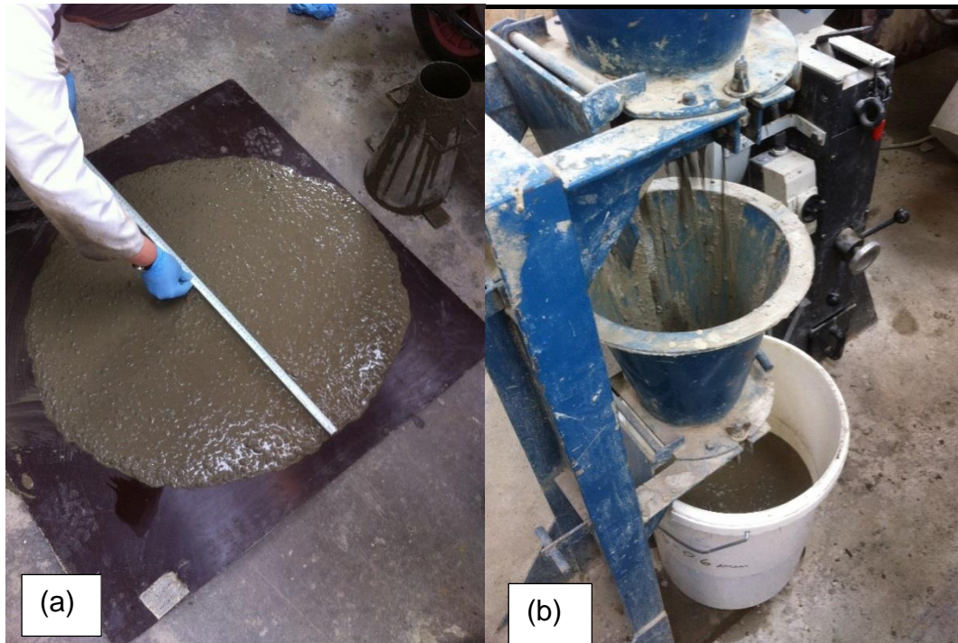
Figure 3-4 Viscosity and filling ability of SCC mixes using (a) slump flow test (b) V-funnel test.
