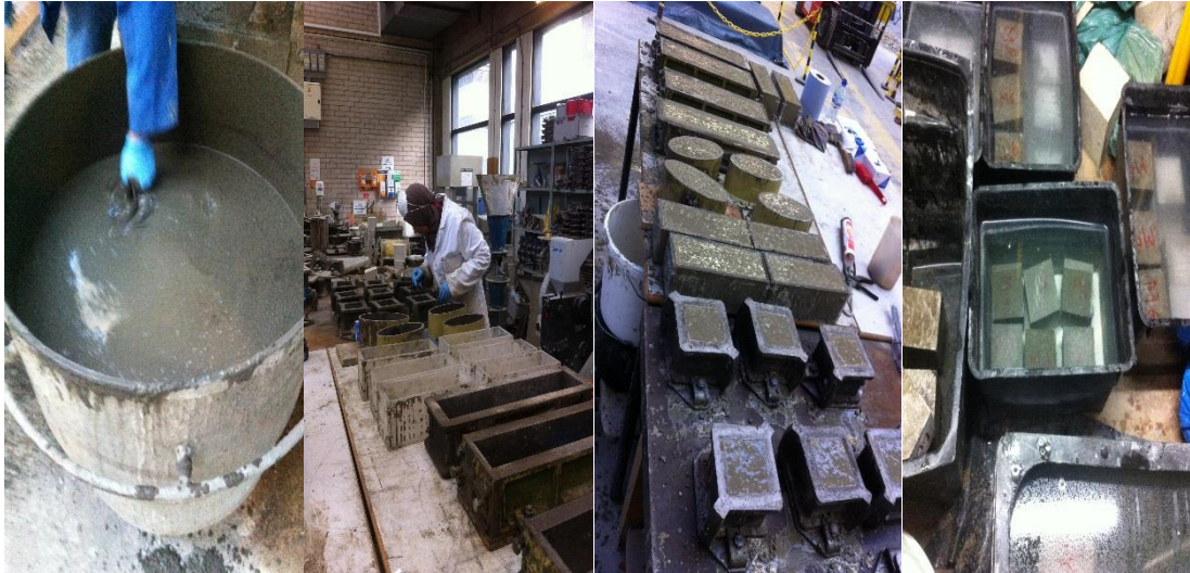
Figure 3-3 Mixing, preparing, casting and curing procedure.
