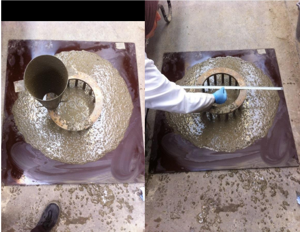
Figure 3-5 Passing ability of SCC mixes using J- ring test.
