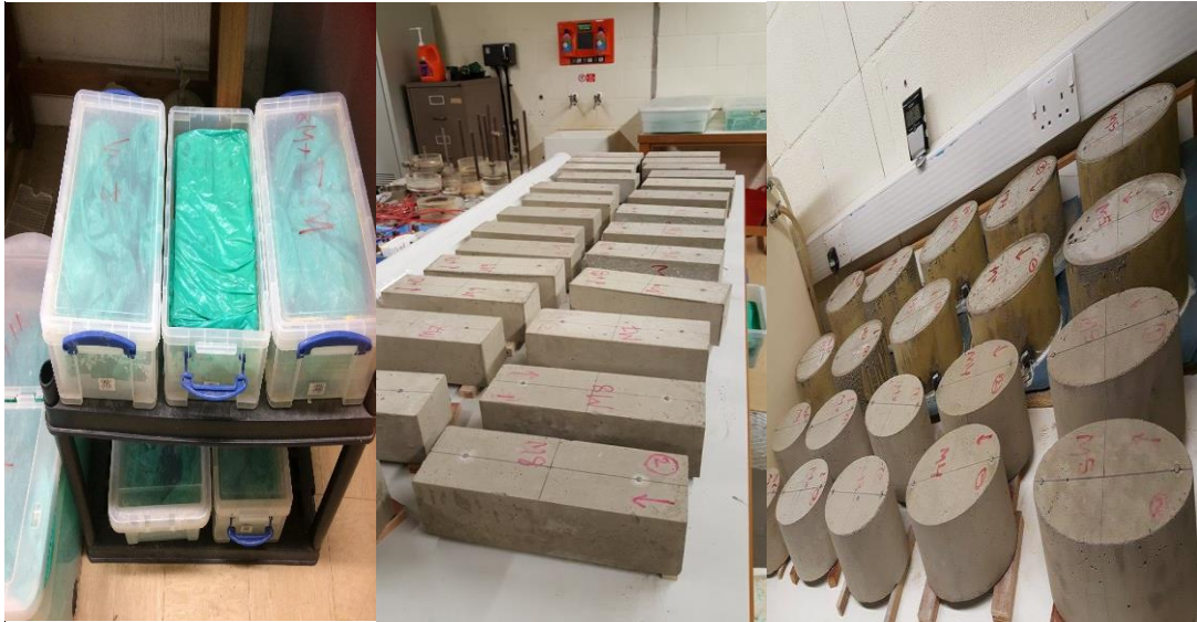
Figure 3-9 Free and confined drying shrinkage strain curing specimens.
