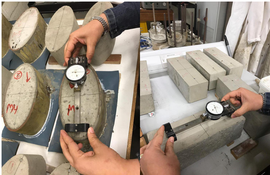
Figure 3-8 Free and confined drying shrinkage strain measurements
