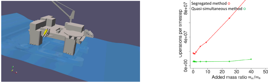
Figure 5: Free-fall life boat being launched (left). The computational effort required per time step for the FSI coupling (right).
