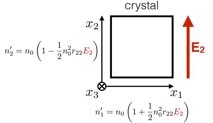
**Fig. 1** The two principal axes of an electro-optic lithium niobate ( $\text{LiNbO}_3$ ) crystal for the case of an electric field  $\mathbf{E}_2$  applied along the axis  $x_2$ . Light is in our case propagating along axis  $x_3$ .
