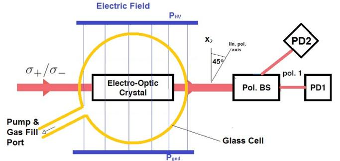
**Fig. 7** Modified setup from Fig. 3.1. The  $\text{LiNbO}_3$  crystal is centered in a spherical glass bulb which can be evacuated and filled with different gases.
