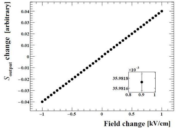
**Fig. 3** Response to an external electric field change for a  $\text{LiNbO}_3$  crystal (Y-cut Z-propagation). The electric field is ramped between  $-1$  kV/cm and  $+1$  kV/cm in square steps of  $50$  V/cm every  $6$  s. The obtained resolution for electric field measurements is  $\delta E > 4(1)$  V/cm. (The insert shows an example of a data point at an enlarged scale.)
