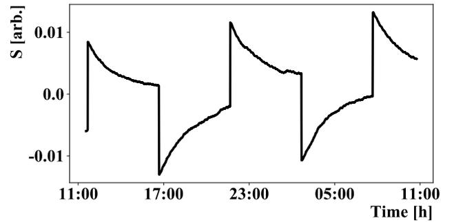
**Fig. 13** Example of the response of the integrated sensor to an electric field which was externally applied in a step function. The electric field was switched between the states 0 V/cm and 1 kV/cm every 5 hours. The signal decay time constant is  $\tau_s = 1.7(1) \text{ h}$ .
