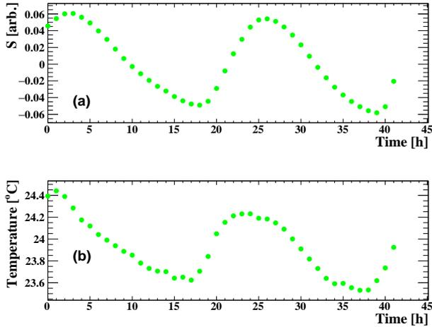
**Fig. 4** Recording of electric field sensor signals in air averaged over 1 h periods (a) and the ambient temperature (b) over a period of 45 h. During every 1 h period a constant electric field was applied externally to the crystal for 0.5 h and thereafter, it was turned off for 0.5 h. Environmental temperature changes caused a correlated variation of the signal  $S$ . The effect has been exaggerated by allowing for rather large temperature fluctuations.
