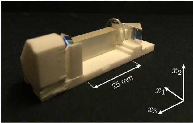
**Fig. 12** Photograph of the integrated electro-optic electric field sensor. The optical fibers connecting to a light source and to two photo-diodes are not shown. Those are attached to the holes visible on the left side of the Macor substrate.
