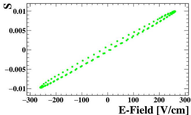
**Fig. 6** Sample of a phase shift measurement between a sinusoidal electric field with a period of 3600s applied to the  $\text{LiNbO}_3$  crystal in Xe/He gas mixture (see also Fig. 10) and the electro-optic response  $S$  over a period of 1 h. The phase shift of 85(5) mrad between both signals yields  $\tau_c^\phi = 1.9(1)$  h.
