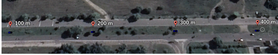
Figure 11: CooPS absolute position validation. The landmarks 100, 200, 300 and 400 m are the corresponding ground positions from RSU_A . The errors are acquired from the comparison between CooPS estimation positions and Google Earth map positions (figure produced using Google Earth).
