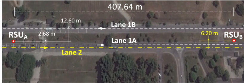
Figure 8: Experimental scenario used for CooPS evaluation performance. Three separate road stretches were used, Lanes 1A, 1B, and 2. We used two fixed road-side units: RSU_A and RSU_B (figure produced using Google Earth).
