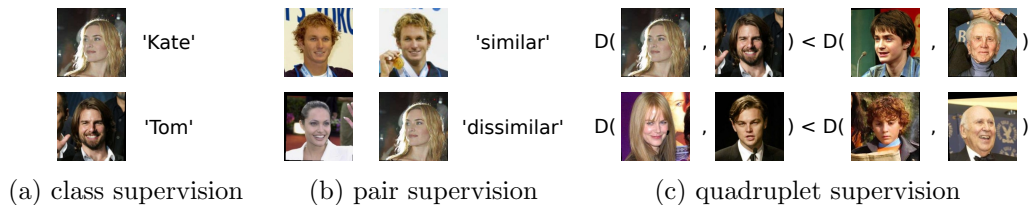
Figure 1: Different types of supervision for metric learning illustrated on face image data taken from the Labeled Faces in the Wild dataset (Huang et al., 2012).
