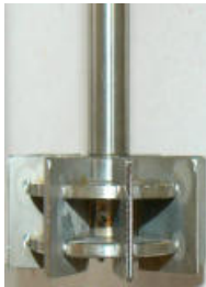
Hollow self-inducing impeller
