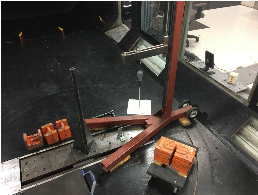
Figure 3.4: Dumbbell Loading in Lift
