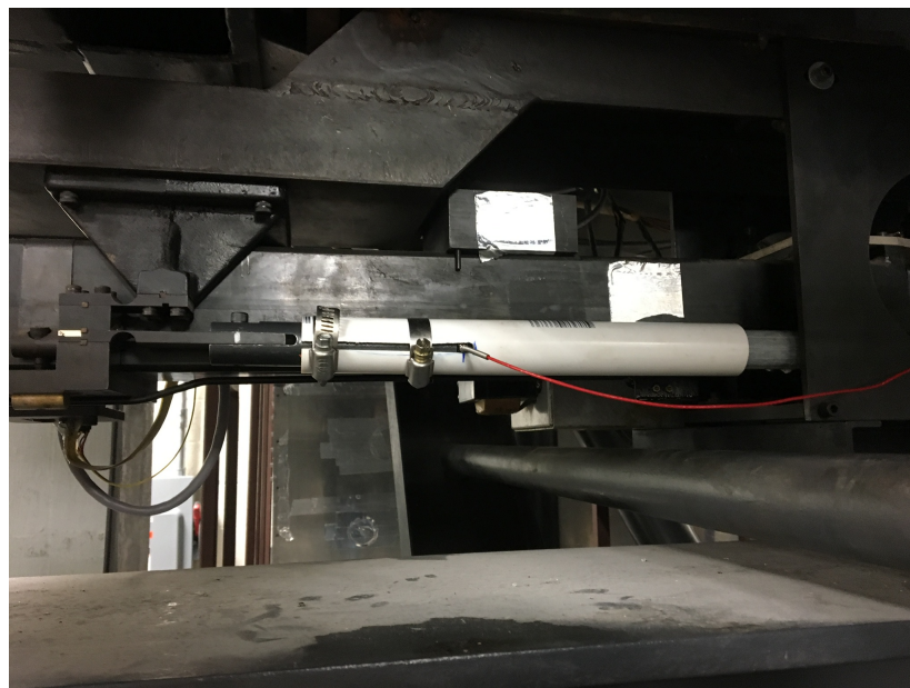
Figure 2.14: Pitch Pushrod Brace Installed, MKIb design
