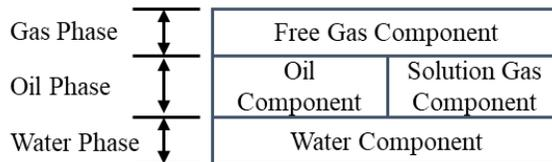
**Figure 2.3 Distribution of components among phases in black-oil fluid (redrawn from (Ertekin et al. 2001))**
