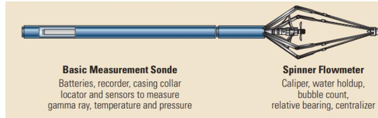
**Figure 1.1 Typical production logging tool (reprinted from (Davaranah et al. 2017))**
