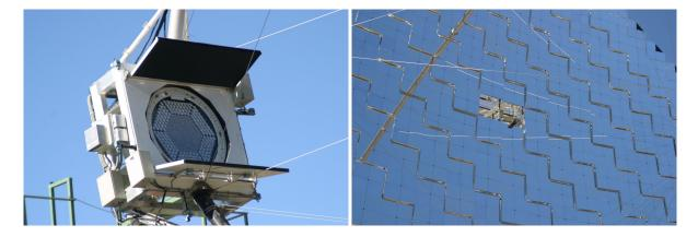
Figure 3.7: Left panel: An image of one of the MAGIC cameras. Right panel: An image of the MAGIC I mirror panels. Images taken from https://magic.mpp.mpg.de/.
