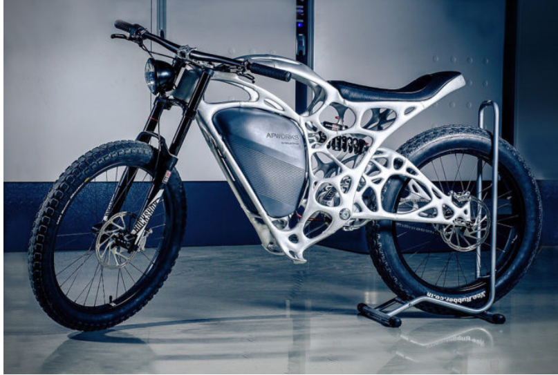
Figure 1.1: Light Rider™ is the world's first additively manufactured motorcycle weighing only 35 kilograms
