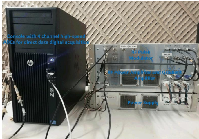
Fig. 24 The one-channel transmitting and four-channel receiving broadband NMR spectrometer.
